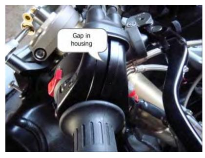
If you have a gap in the housing after it is bolted together more adjustment is needed on the acceleration cable
